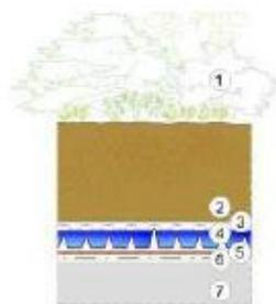
(1)Vegetation, (2)Growing media, (3)VLF 150/200 filter layer, (4)DiaDrain-40H, (5)VLU 300/VLS 500 mechanical protection layer, (6)Root resistant waterproofing membrano, (7)Root construction
